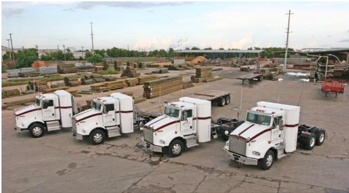
The new trucks are 2015 Kenworth T800's powered by Cummins Westport's new ISX12 G 400 engine, which is a 12 liter engine rated up to 400 horsepower and 1,450 lb-ft of torque. Building Products Plus is one of the first companies to have the 12 liter CNG-fueled trucks in operation.
